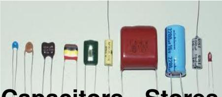
**Capacitors - Stores electrons in an electric field**
